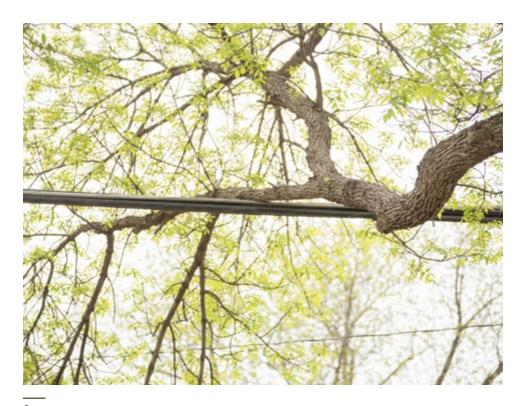
Managing vegetation along high-voltage power lines is a top priority for Chelan County PUD. Trees and power lines do not mix. Trees contacting power lines are a leading cause of power outages, can start fires and are a public safety hazard.
