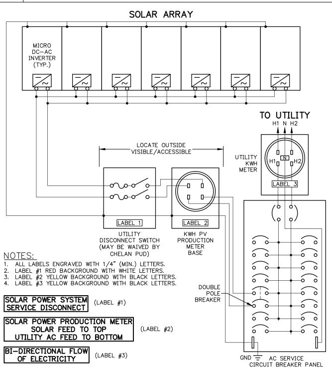
NOTE: THIS DIAGRAM SHOWS ELECTRIC METERING REQUIREMENTS THAT COMPLY WITH CHELAN COUNTY PUD INTERCONNECTION STANDARDS FOR CUSTOMER-OWNED RENEWABLE POWER GENERATION SYSTEMS. THIS DIAGRAM MAY NOT SHOW EVERYTHING NEEDED TO MEET MINIMUM ELECTRIC CODE REQUIREMENTS. CHELAN PUD WILL NOT INSTALL AN ELECTRIC METER UNTIL THE INSTALLATION HAS BEEN APPROVED BY
