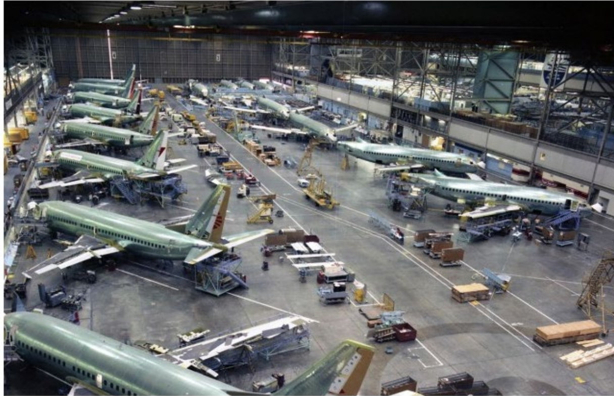
The Boeing 737 Assembly line number 1 at Renton in the 1980s as the 2nd generation 737-300/400/500 series was taking over for the first generation 737-200 Classic. Image Courtesy: Boeing
