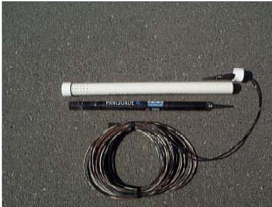
Figure 4-4: MiniSonde Temperature Logger Used for Fixed and Mobile Monitoring
