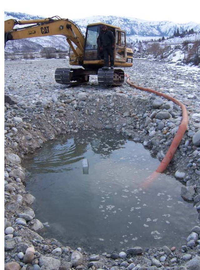
Photograph 10 – STA 18+50 Falling Head Test
