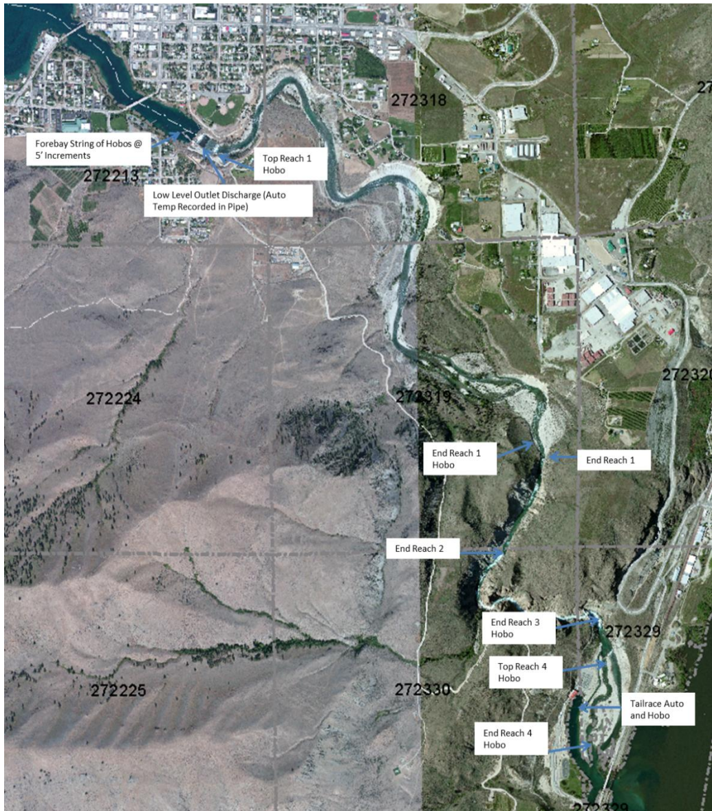
Figure 7. Chelan River in-stream temperature monitoring stations
