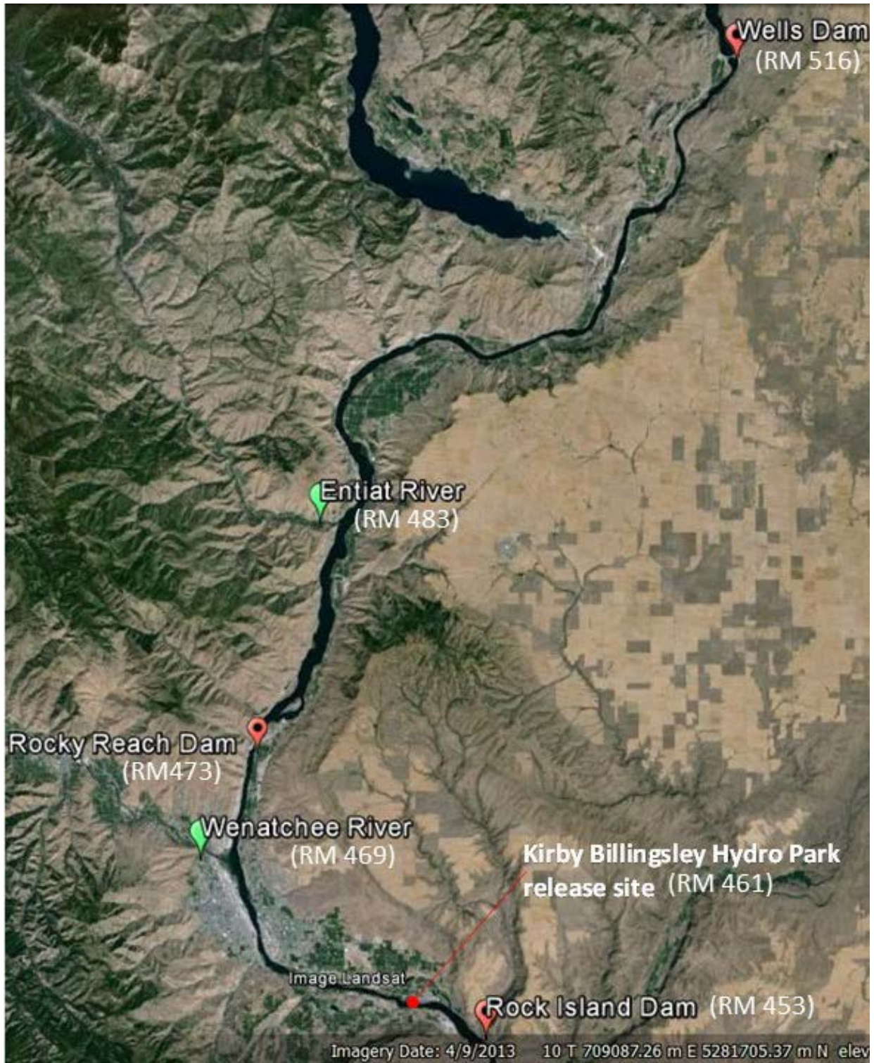
Figure 4. Full-duplex PIT tag detection sites are located at Rock Island, Rocky Reach, and Wells dams as well as tributary detection sites in the Wenatchee and Entiat rivers. Detections of tagged lamprey released for the study were queried using the PTAGIS website ( www.ptagis.org ).
