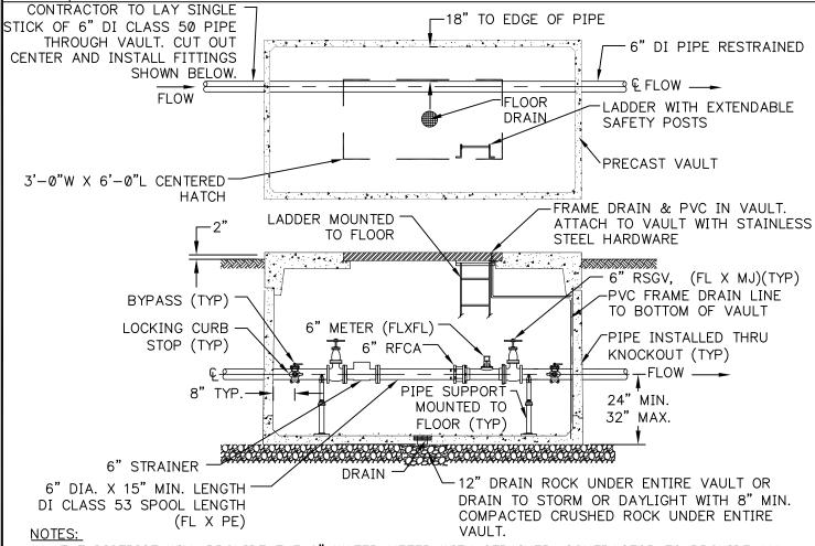
THE DISTRICT WILL PROVIDE THE 6" WATER METER WITH STRAINER. CONTRACTOR TO PROVIDE ALL OTHER MATERIALS. MATERIAL COSTS BORNE BY THE CUSTOMER.
