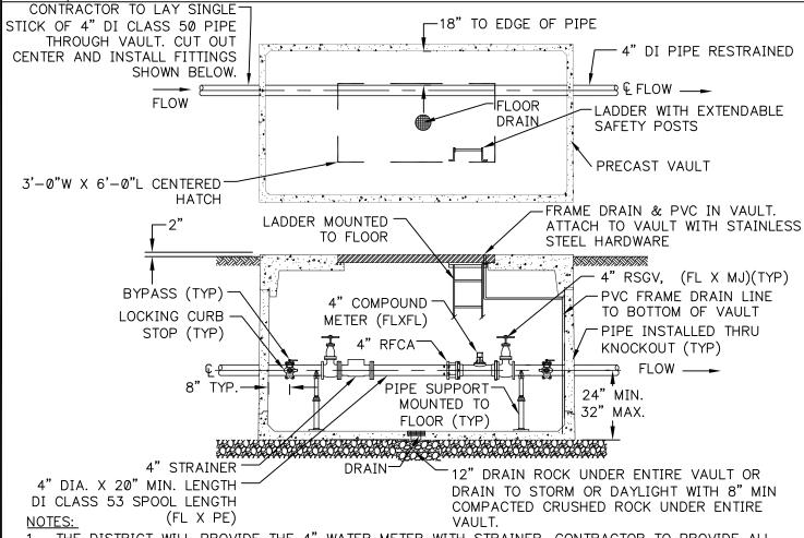
1. THE DISTRICT WILL PROVIDE THE 4" WATER METER WITH STRAINER. CONTRACTOR TO PROVIDE ALL OTHER MATERIALS. MATERIAL COSTS BORNE BY THE CUSTOMER.
