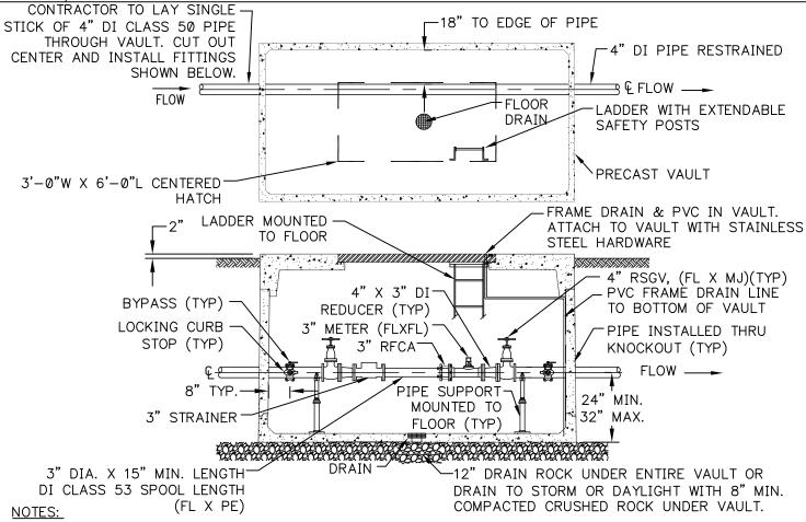
1. THE DISTRICT WILL PROVIDE THE 3" WATER METER WITH STRAINER. CONTRACTOR TO PROVIDE ALL OTHER MATERIALS. MATERIAL COSTS BORNE BY THE CUSTOMER.
