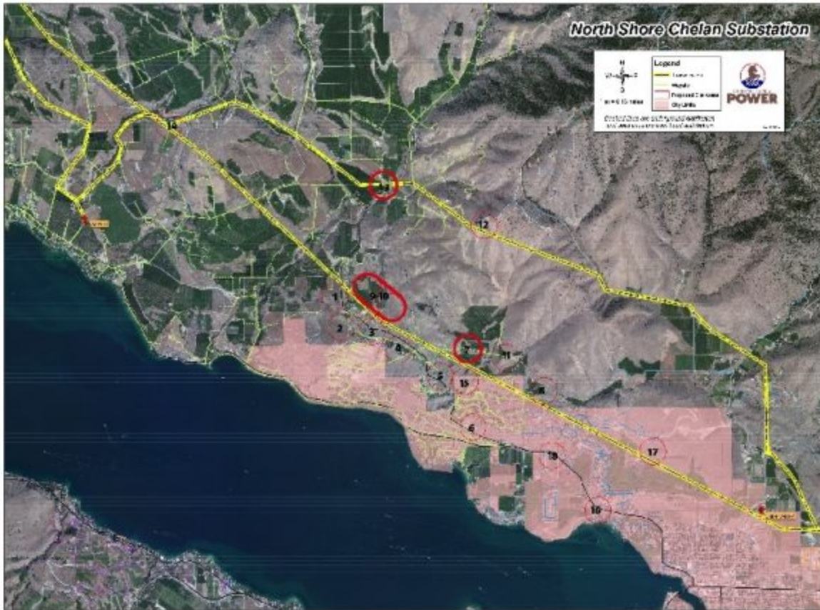
Chelan PUD map showing all proposed locations for a North Shore substation, and the three locations that are considered the prime areas close to existing transmission lines. (Image courtesy of Chelan PUD)
