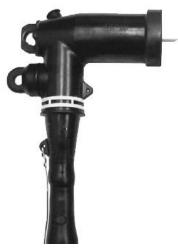
Application: The 200 amp loadbreak separable elbowbushina connector is suitable for connecting URD underground cable to URD transformers and switchgear. It provides а arounded. deadfront. submersible cable connection. Loadbreak and load make operations require the aid of a live-line tool (shotgun stick with elbow puller).
