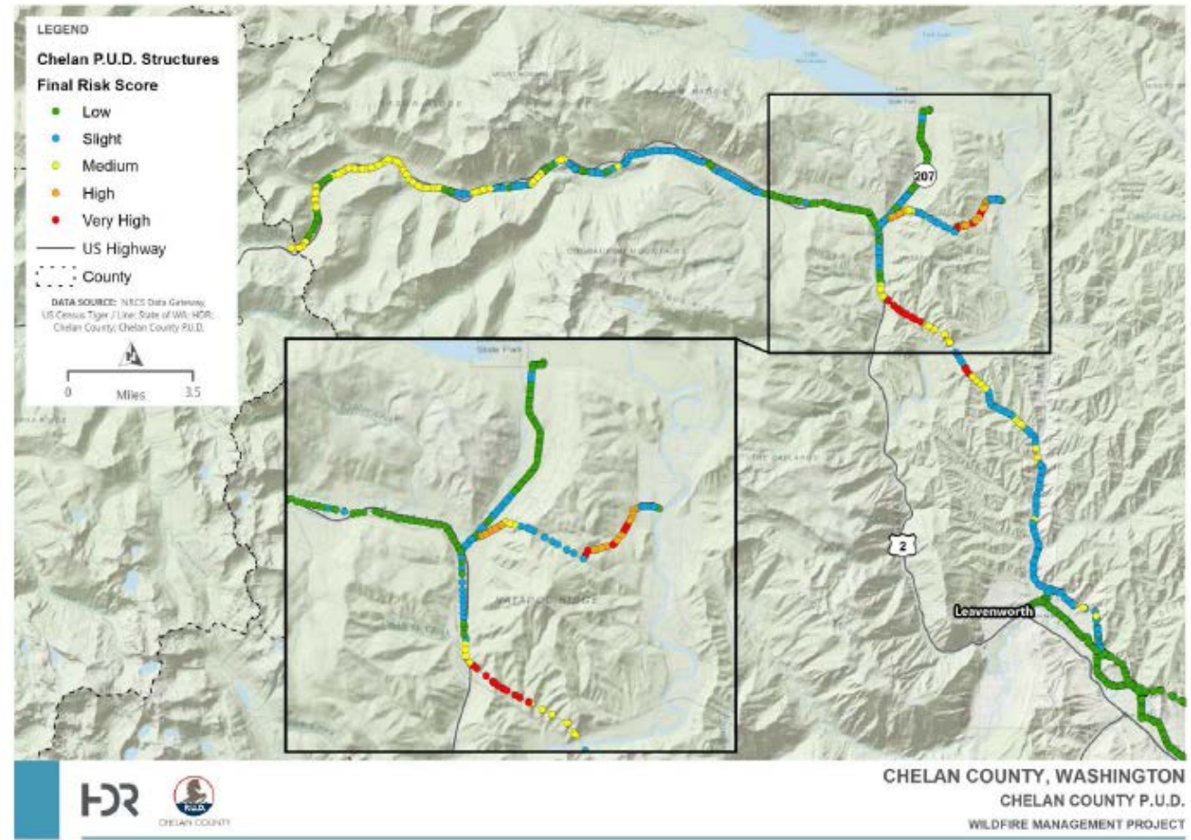
Figure 14. Map showing the structure-by-structure final risk score associated with the northwestern portion of the district's serv
