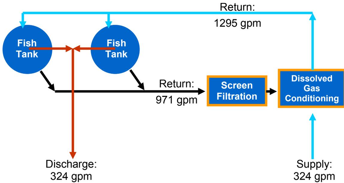
**Figure 1.** Schematic of the partial water reuse system installed at the Eastbank Hatchery in Wenatchee, WA. The system includes two circular 30-ft diameter dual-drain tanks, microscreen filtration and gas conditioning of influent and recirculating water.
