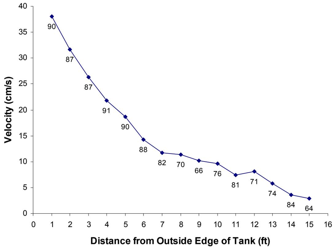
**Figure 3.** Circular tank velocity profile measured in late October, 2009. Velocities ranged from approximately 38 cm/s at the outside wall to less than 5 cm/s near the center of the tank. Numbers appearing beside each data point represent the resultant angle of measurement (relative to the 90-degree tangent at the tank wall).
