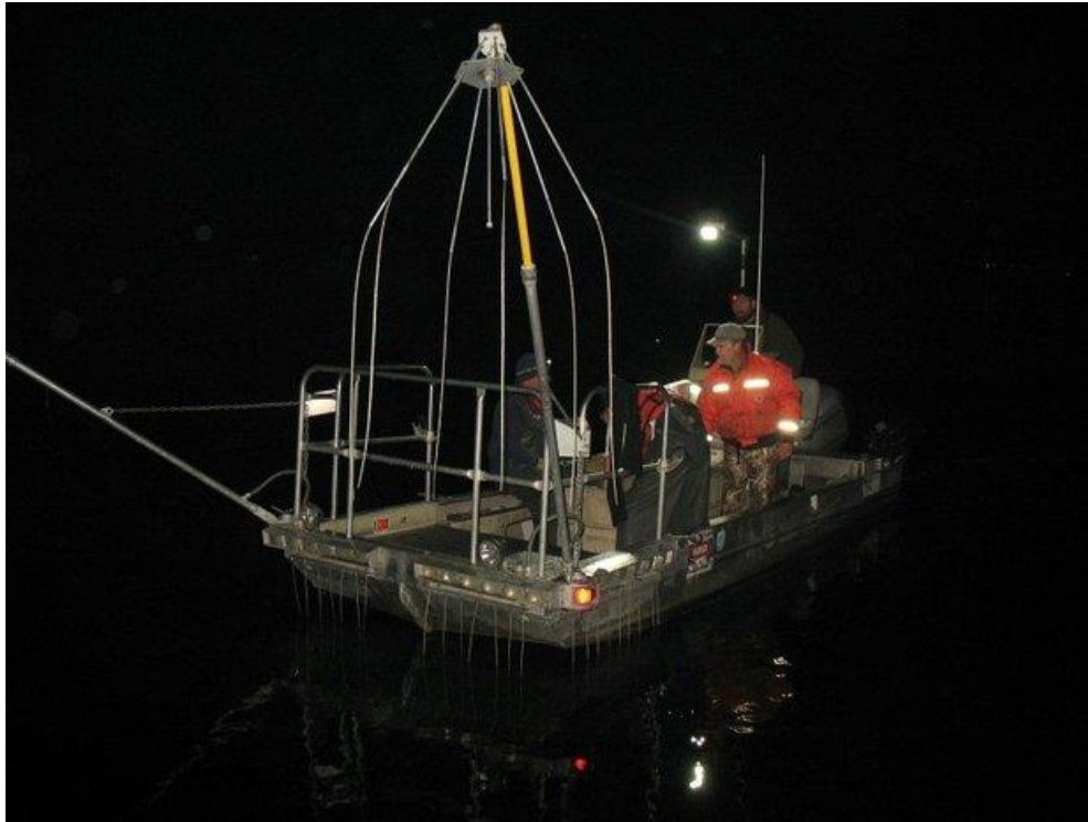
Figure 3. LLRT electrofishing boat preparing to commence shocking run at a prescribed site during the 2012 survey. Whisker-like booms in the foreground are lowered into the water prior to starting the on board generator.
