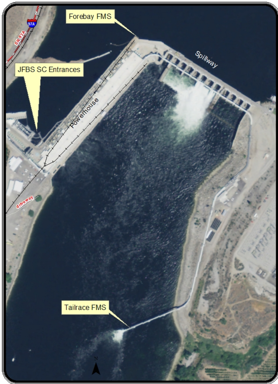
Figure 2.1. Location of the forebay and tailrace FMSs, and the JFBS SC entrances
