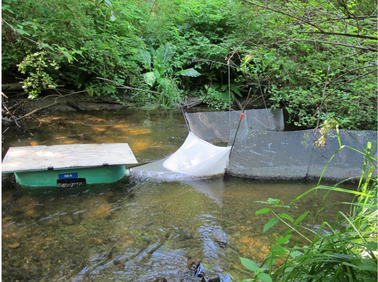
Figure 3: Photograph of live downstream lamprey trap.
