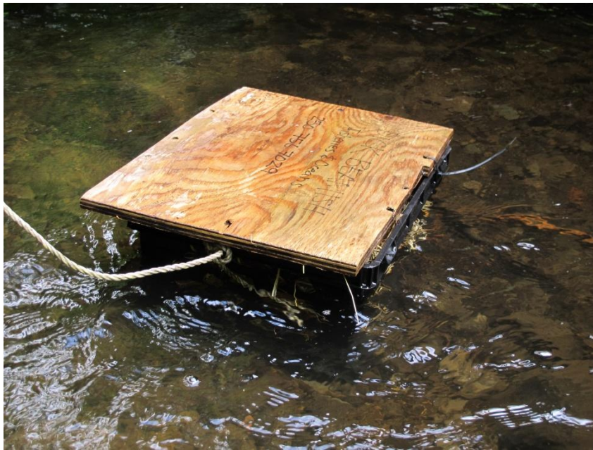
Figure 2: Photograph of milk crate lamprey trap.
