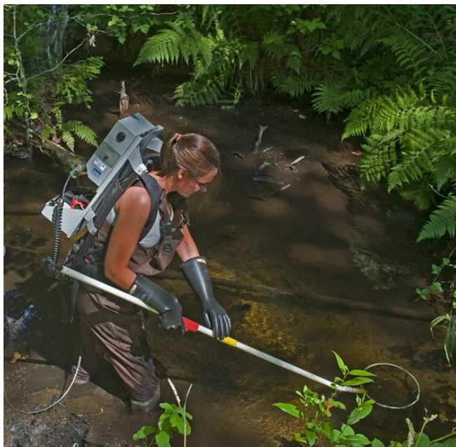
Figure 4: Photograph of electroshocking for lamprey in British Columbia.
