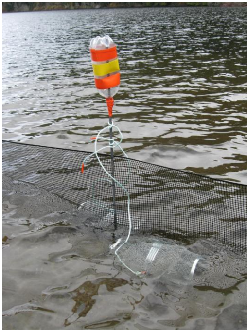
Figure 1: Photograph of lamprey weir with wire mesh trap.
