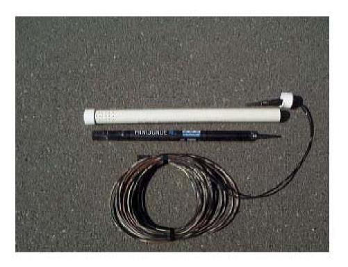
Figure 4-4: MiniSonde Temperature Logger Used for Fixed and Mobile Monitoring
