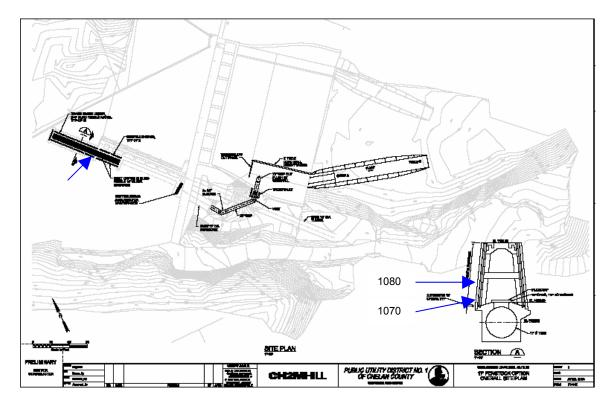
Figure 4-1: Potential Outlet Structure Using the Existing Intake for the 17-Foot Future Power Tunnel with Location of Fixed Temperature Monitoring Site (Arrows)
