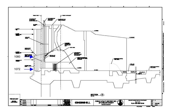
Figure 4-3: Location of Fixed Temperature Monitoring Site (Arrows) at Potential Outlet Structure at the Existing Spillway Trash Sluiceway
