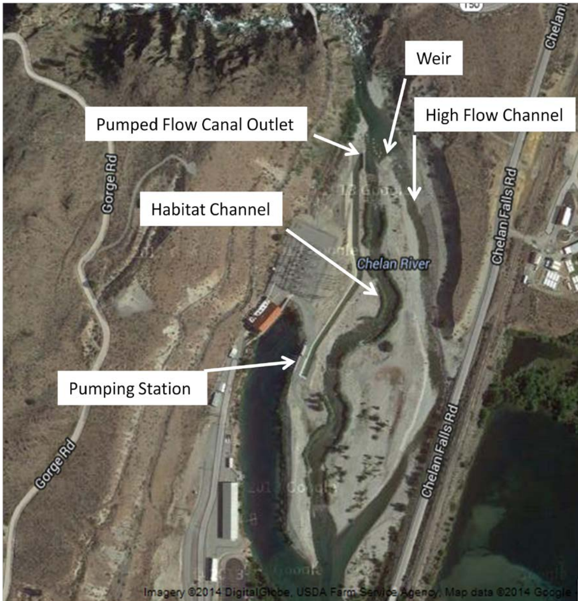
Figure 4. Chelan River Reach 4 showing habitat channel and structures.
