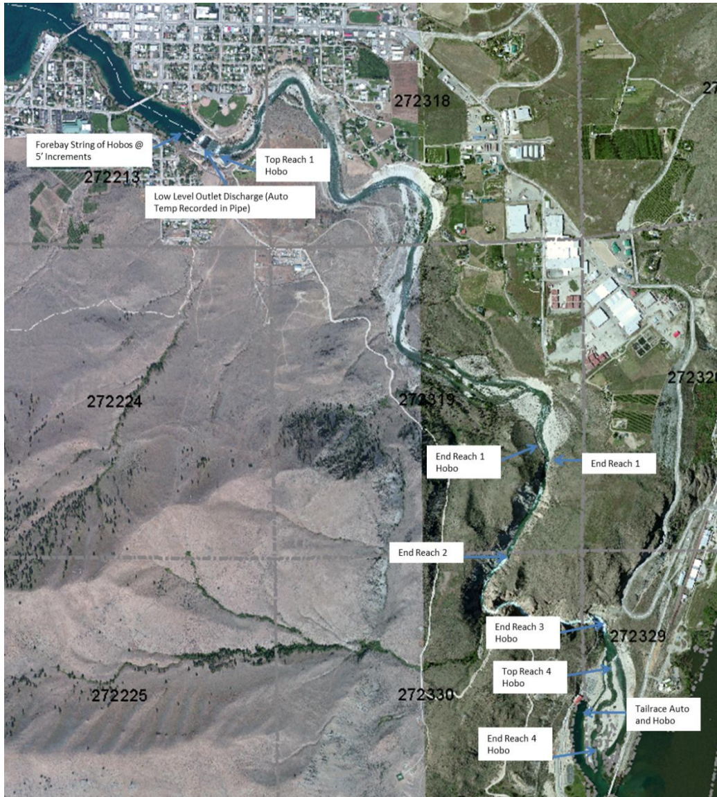
Figure 7. Chelan River in-stream temperature monitoring stations
