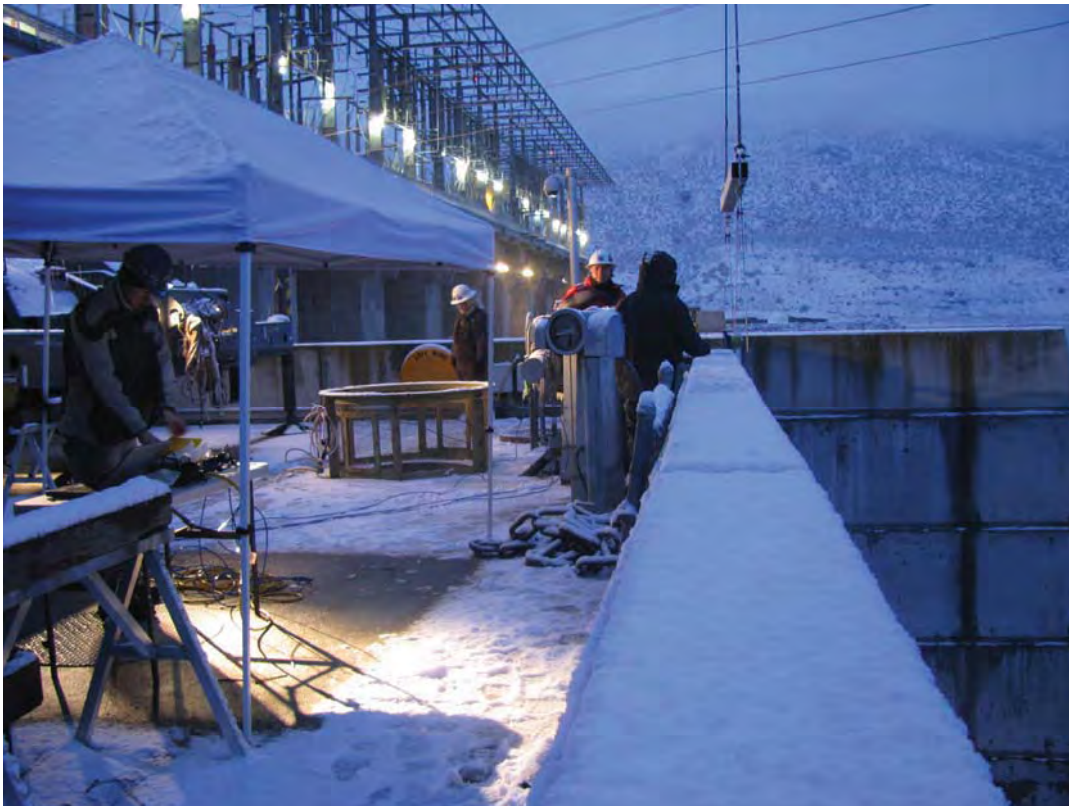
Photo 8: The high tailwater condition testing was concluded at dawn on March 2nd. The ADVs were controlled via a laptop under the tent shown on the left. (Photo by NHC)
